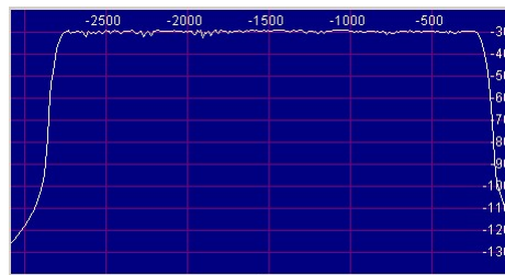
Filter Characteristics 6dB Bandwidth 2587 Hz, 60dB Bandwidth 2756 Hz Shape Factor ~1.06
